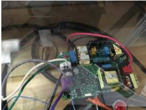
(Picture: Sample LED Driver under Bench test)
